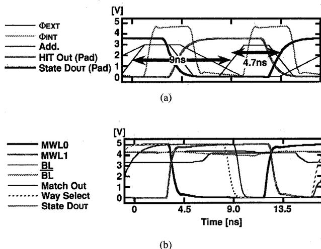
Fig. 8. Simulated waveforms of a Tag look-up cycle.
