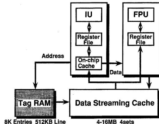
Fig. 1. Data streaming cache architecture.
