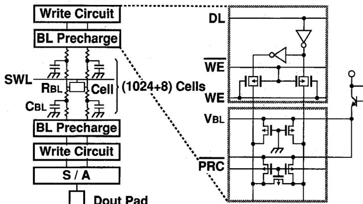
Fig. 7. Doubly placed precharge and write control circuit.
