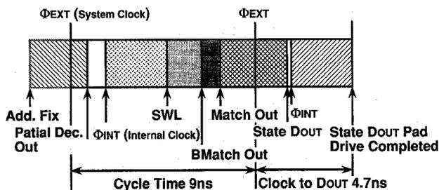
Fig. 9. Distribution of delay time in a Tag look-up cycle.
