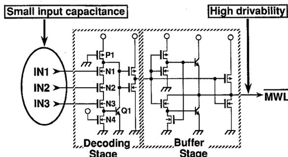
Fig. 4. Single PMOS load BiCMOS main decoder.
