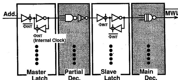
Fig. 3. Pipelined partial decoding scheme.
