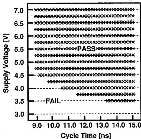
Fig. 11. Schmoo plot. The 9.0-ns cycle operation is achieved at the supply voltage of 5.0 V.
