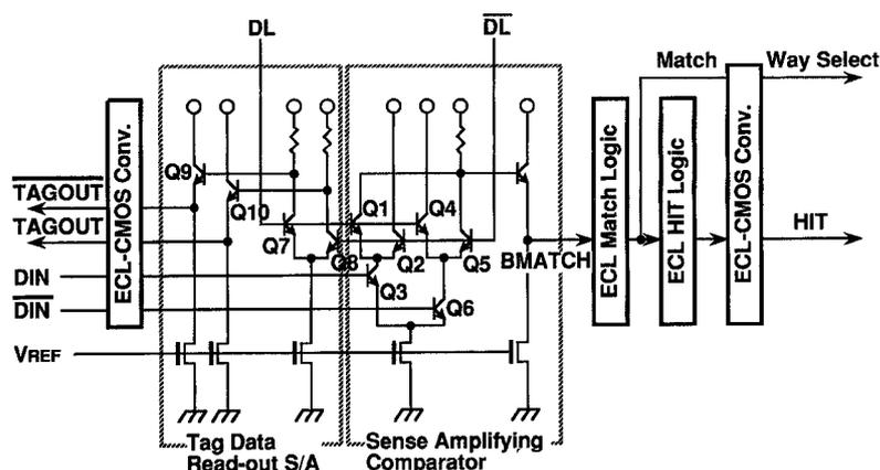
Fig. 5. Sense-amplifying comparator (SAC).
