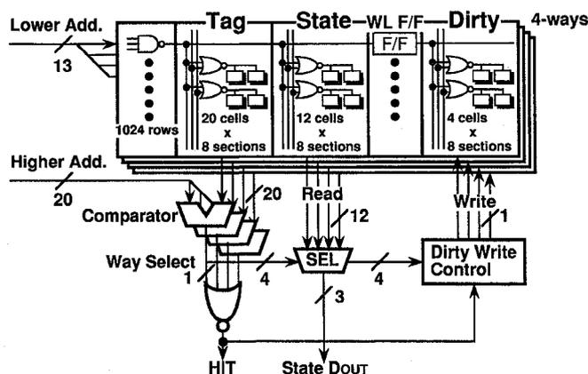
Fig. 2. Memory core architecture for Tag look-up operation.
