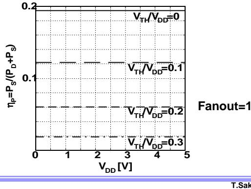
Fig.14 The change of the short-circuit power dissipation with scaling
