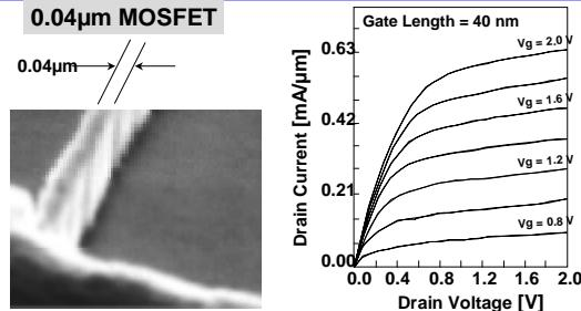
Conventional I-V curve at 0.04 μm (Even down to 0.014 μm)
