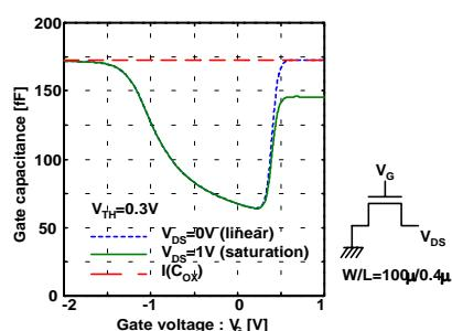
Fig.15 Voltage dependent gate capacitance effect
