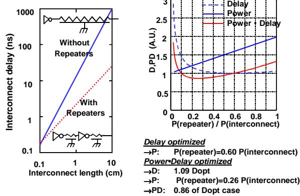
Fig.43 Delay and power optimization from repeaters
