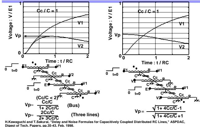
Fig.47 Coupling noise in RC bus
