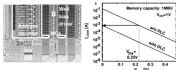
Total subthreshold leak of 1Mbit SRAM. At 1V VDD, VTH of the dormant cell is 0.25V while that of the active cell is 0V, keeping the total leakage power at 0.9mW.
