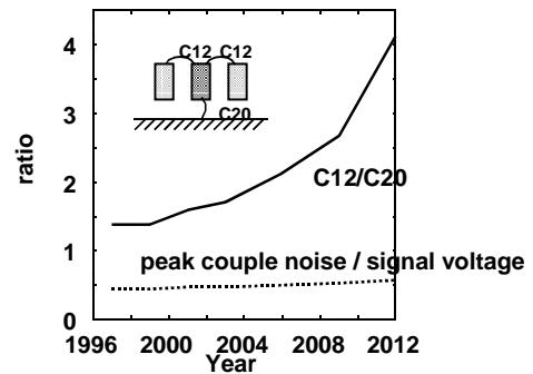
Fig.46 Capacitive coupling noise
