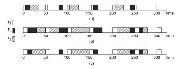
Figure 2. A schedule for the example task set. (a) When tasks always run at their WCETs. (b) When tasks always run at their WCETs on a processor with the speed lowered by half. (c) When the execution times of some task instances are smaller than their WCETs.
