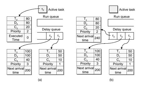
Figure 4. The status of queues and the information associated with each task (a) at time 160 and (b) at time 180.
