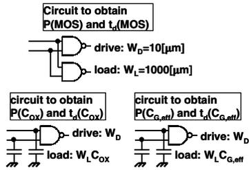
Fig. 6 Circuit to simulate effect of substituting real MOS gate capacitance by  $C_{OX}$  and  $C_{G,eff}$
