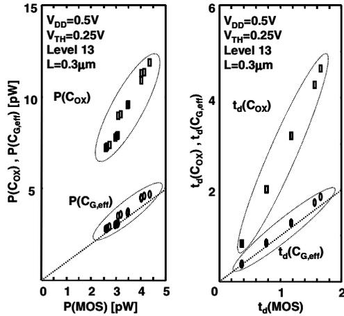
Fig. 7 Dynamic power dissipation and delay of 4-bit counter
