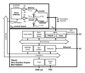
Figure 6. A block diagram of the hardware platform.
