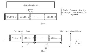
Figure 2. Application slicing. (a) Slicing structure. (b) Scheduling of slices.
