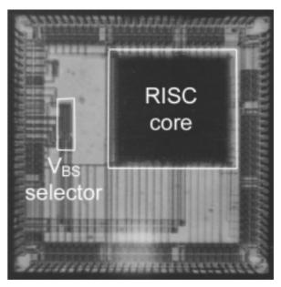
Fig. 8 Microphotograph of RISC processor
