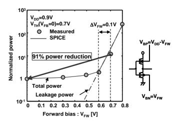
Fig. 10 Delay and power of  $V_{\text{TH}}$ -hopping with positive back-gate bias
