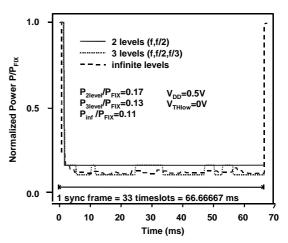
Fig. 4 Power transition of V<sub>TH</sub>-hopping
