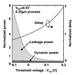
Fig. 1 Power and delay dependence on  $V_{TH}$
