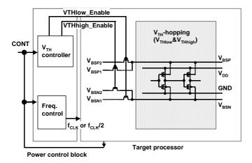
Fig. 3 Schematic diagram of V<sub>TH</sub>-hopping
