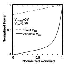
Fig. 2 Power dependence on workload
