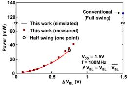
Fig.3 Write power consumption of bit lines versus bit line swing  $\Delta\,V_{\text{BL}}$
