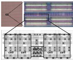
Fig. 6 Microphotograph and cell layout
